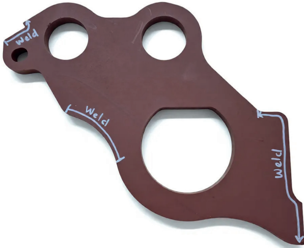
Front plate weld area.
