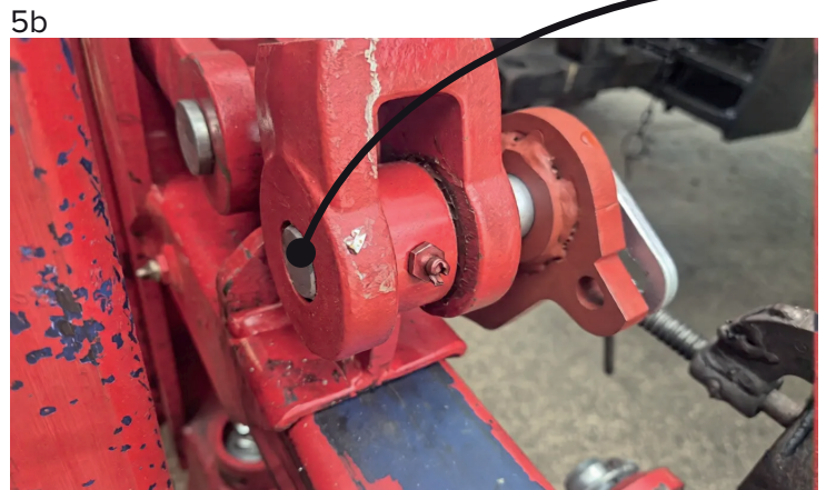
Pin pushed through side tilt ram clevis.
